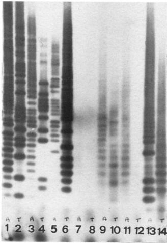
Fig. 2.- MVR-PCR patterns after non-radioactive hybridization of an agarose gel; the amplification condition number 2 of Materials & Methods were used.
